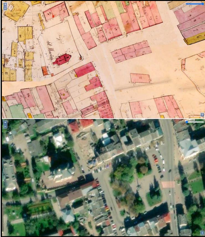
Two views of the map overlay: the georectified 1846 cadastral sketch (top) and the satellite image of the modern town (bottom). Both show a portion of the town square and a church, labeled as St. Maria on the top map.
